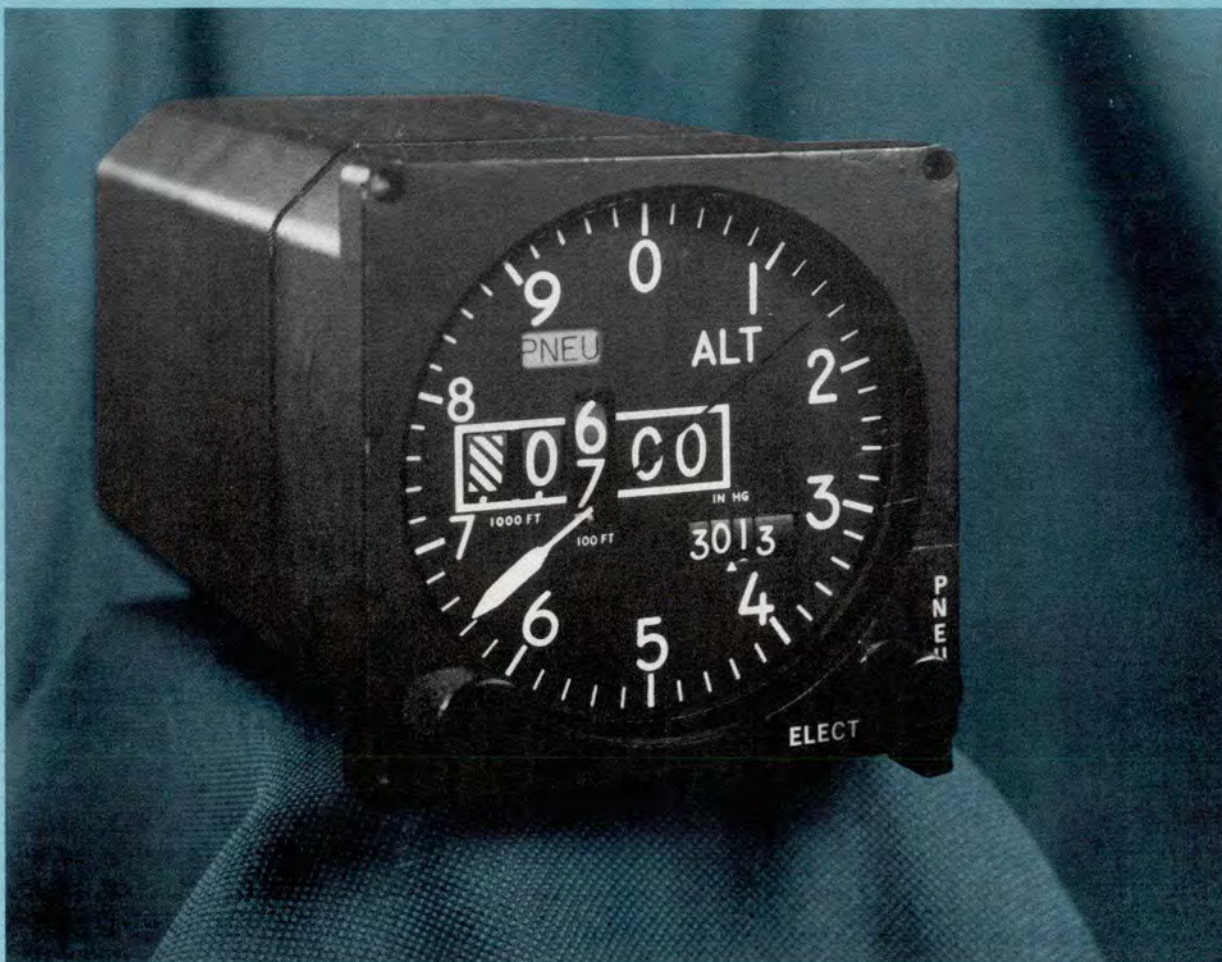
Figure 1—AAU-34 counter drum pointer altimeter.
